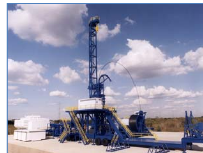
COIL TUBING INJECTION RIG
