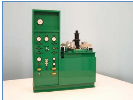
VALVE TESTING CONSOLE
