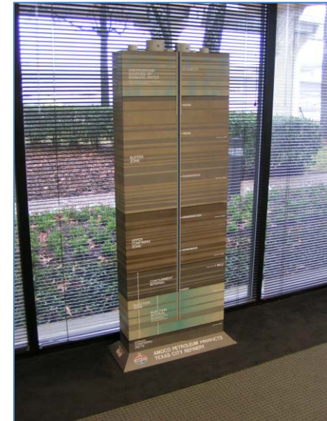
SUBSURFACE INJECTION WELL MODEL
